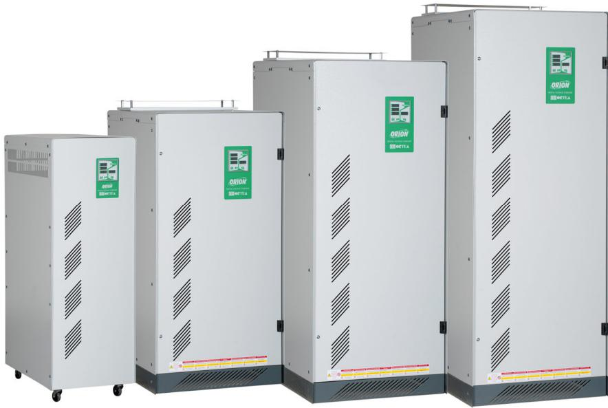
The regulation in the ORION Y stabilisers is independent on each phase. These stabilisers are used with three-phase loads and single-phase loads with 100% unbalance with unbalance input rated voltage and are suitable even in case of non-symmetric mains. In this configuration, **the voltage stabiliser requires the neutral wire presence**. It can also operate without neutral wire by adding a proper equipment ( $\Delta/zn0$  or  $\Delta/Y$  isolating transformer or neutral inductance).
